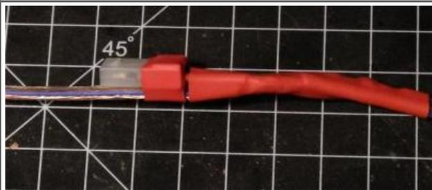
Shrink tube (5/8") or tape the connection. Use the appropriate color tape or tube.
