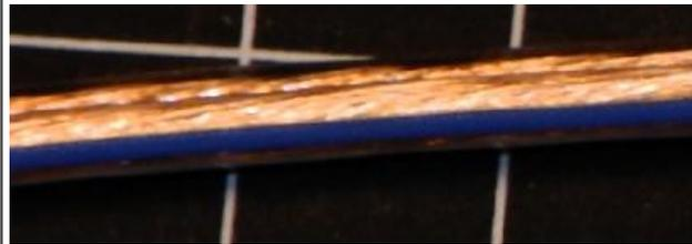
Note that one side of the cord has a blue line in this case. This side is the Power/Blue side. That obviously makes the other side the Neutral/White side. (other wire uses other indicators)
