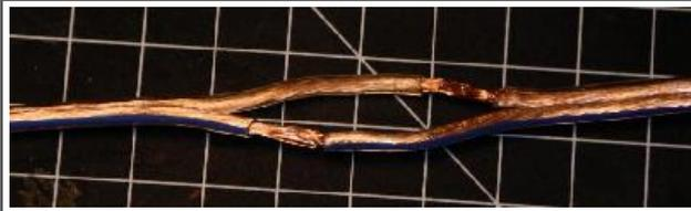
Starting at 2 ft, strip a short section of each wire, offset as shown, every 4 feet. About 1/2 inch is more than enough.
